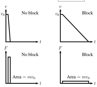
The same idea is used in cars with crumple zones, collapsible steering columns and airbags.
