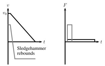
A timid sledgehammer wielder who does not hit the concrete block hard enough to fracture it can be very dangerous
